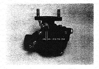
With this spring tension against the governor lever, adjust the throttle rod to provide .010 to .060 between the carburetor bellcrank and wide open stop.
