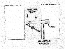
The governor throttle valves are offset in the throttle bore so that the combined force of the manifold vacuum and the fuel/air flow through the bores has greater effect on the larger, upstream area of the valves.
