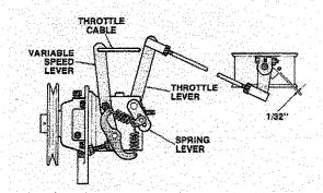
The belt driven governor must be driven by the engine at a fixed ratio. The governor pulley size and belt arrangement are determined by the engine application and the speed at which it is to be governed.
