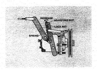
The third type of spread adjustment is the eye bolt type. Adjustment is made with the eye bolt that attaches the spring to the variable speed lever.
